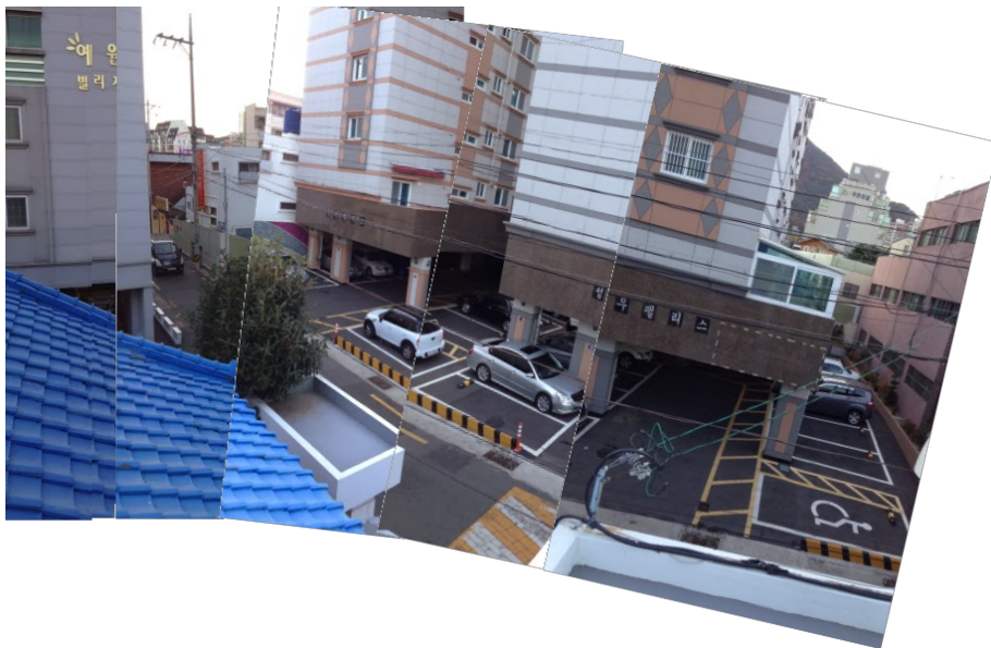
Figure 4: A panograph which is created by using the STANDARD stitching mode for panography or mosaic stitching of the input images. In this case, SIFT is used again for feature detection and feature extraction in the stitching process.
