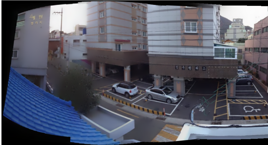
Figure 3: A composite image which is created by using the COMPROMISED stitching mode for seamless stitching of the input images, while using SIFT as main feature detector and extractor in the stitching process.
